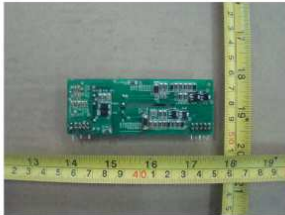
Bottom of driver board
